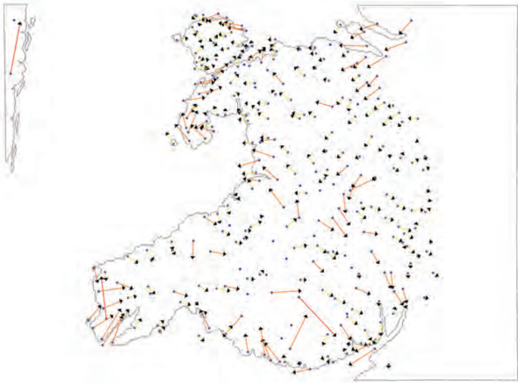
FIGURE 6: GIS map-output using MapAnalyst™ displacement vectors for Cambriae Typus .
